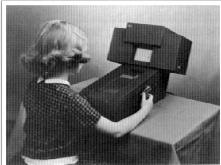
FIG. 1. A recent model of a teaching machine for the lower grades. The machine operates in the principles described in the accompanying article. Material is presented in a window with a few letters or figures missing. The pupil moves sliders which cause letters or figures to appear. When an answer has been composed, the pupil turns a crank. If the answer was right, a new frame of material moves into the window and the sliders return to their home position. If the answer was wrong, the sliders return but the frame remains and must be completed again. (This is a later version of the device described in Skinner's 1954 paper.)
